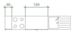
This is the minimum provision for a kitchen. It incorporates worktop on both sides of the cooker and working space both sides of the sinkbowl. Note 300mm is a minimum width and should be made wider where posssible.
