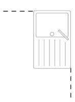
The sink bowl must not be located in a corner. This is an impractical arrangement and because there is no worktop next to the bowl and it is impossible to separate clean and dirty utensils, it also creates a hygiene hazard.
